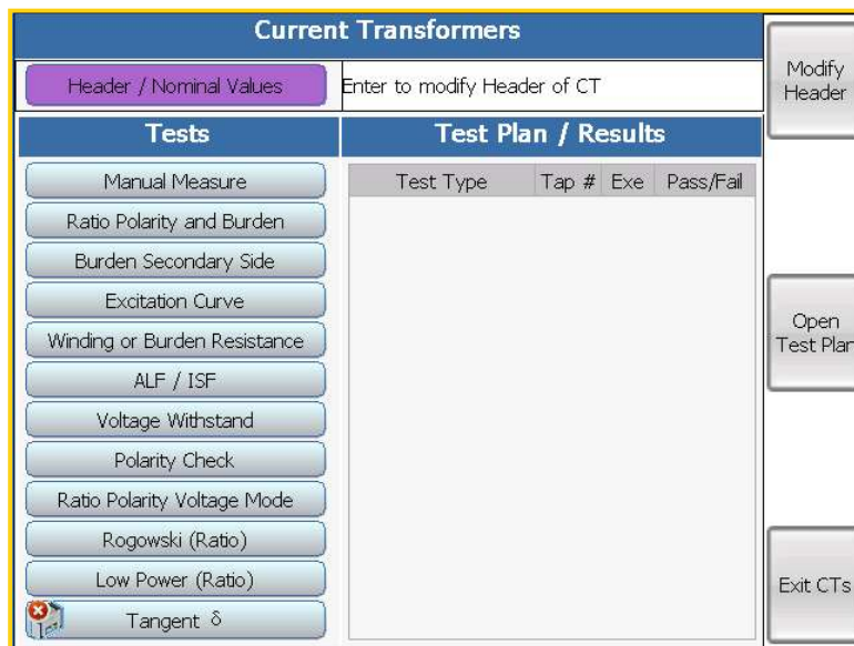
Figure 11 - "Current Transformers" test page (Conventional Type)
