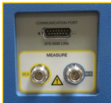
Figure 35 - IN-A (UST-A) and IN-B (UST-B) measurements on the side
