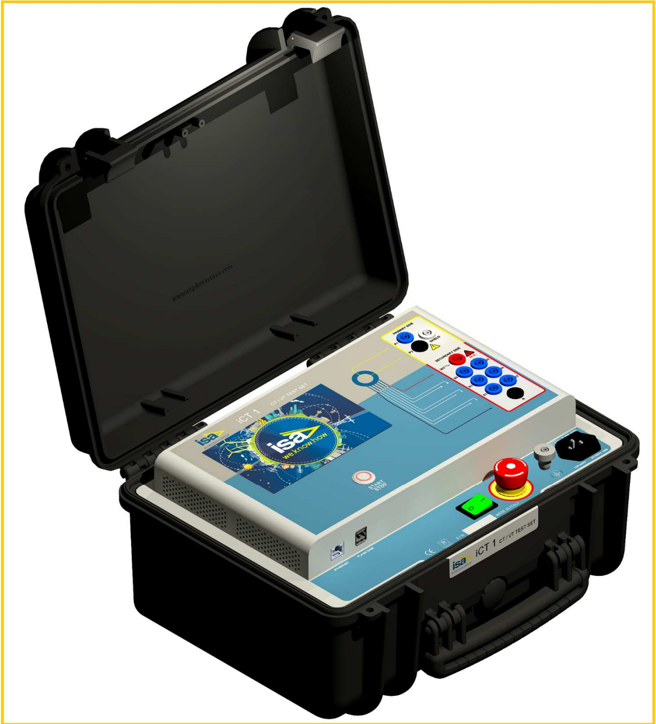
Figure 1-iCT 1 – CT / VT Test set
